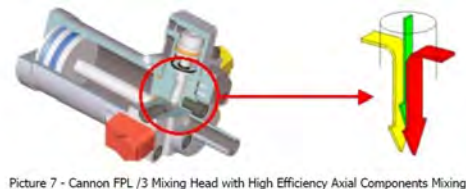
Picture 7 - Cannon FPL /3 Mixing Head with High Efficiency Axial Components Mixing
